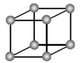
In the primitive cubic unit cell, the atoms are only located on the corners. That means 8 atoms are located on 8 corners of the lattice. Each atom located on the corner contributes 1/8<sup>th</sup> of the original volume of the cell. Since there are total 8 atoms in a primitive cubic unit cell,
